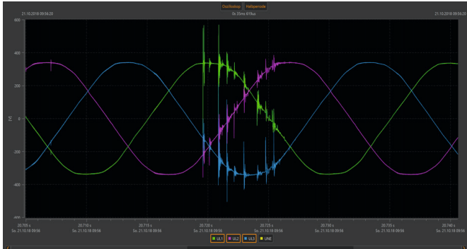
Figure 9: Fast switching transients in an industrial installation, measured with a PQ-Box 200
