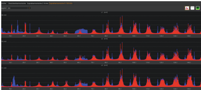
Figure 5: Detection of supraharmonics up to 150 kHz in 200 Hz bands (PQ-Box 300)
