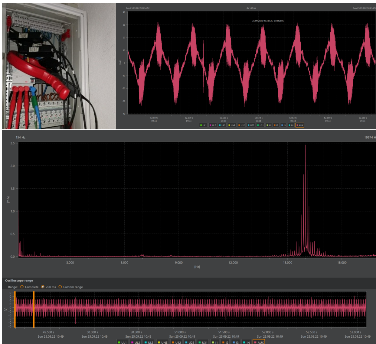
Figure 8: Measurement of residual current at an RCD, including analysis of the fundamental component and supraharmonic currents
